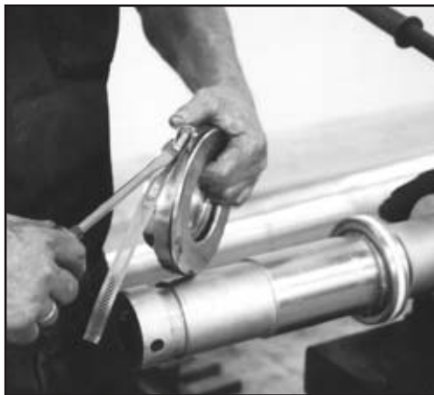
FIG. 120: USE COMPRESSION CLAMP TO REFORM SEAL
