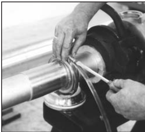
FIG. 119: USE COMPRESSION CLAMP TO REFORM SEAL
