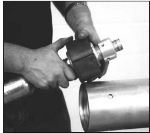
FIG. 76: REPLACE ELASTIC BLOCK
