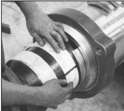
FIG. 106: REPLACE PISTON SEALS
